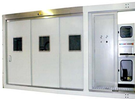
The test bench has been studied for a more efficient internal cleaning of the hoses. Each station is adjustable at will by the operator, the pumps are capable of delivering a total of more than 500 l/min using low viscosity fluids (8 to 10 cst). Has been matched to the function of flushing a circuit for testing pressure up to 700 bar, this allows the bench to have a high functional flexibility able to meet many of the typical requirements of a center of fitting systems.
