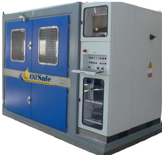
The BASIC PULSE bench for impulse testing of hoses is able to perform testings with "square" wave in accordance with ISO-UNI 6605, UNI ISO 6803, DIN 20 024 and SAE J343d.
