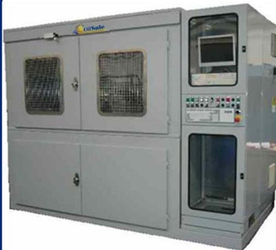
The SUPER DYNAMIC bench for impulse test of hoses is able to perform testings with waves by various forms according to the ISO-UNI 6605, DIN 20 024 and SAE J343d, with spike input according to ISO 6772 or with spike in the final.
